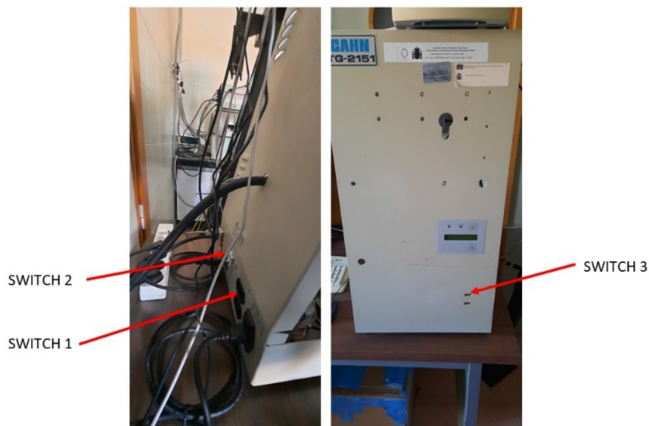
Figure 15: Switches of the furnace
