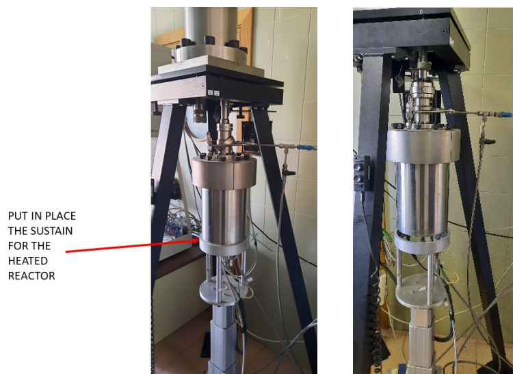
Figure 10: In the left part of the figure it can be seen the PTGA when it is opened (with the support put in place); in the right part of the figure it can be seen the PTGA once it is closed
